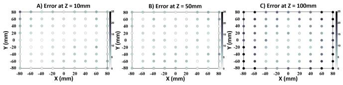
Figure 5. Tracking accuracy is tested in three heights a) 10mm, b) 50mm, and c) 100mm using TMotion. The grayscale indicates the Euclidean distance between the ground truth and our tracking. Origin of the graph represents the center of the magnetometer from mobile device's side. The mean error is 4.55mm in the volume that covers the 5.5'' smartphone, 80mm (x-axis)  $\times$  120mm (y-axis)  $\times$  100mm (z-axis)
