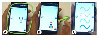
Figure 10. TMotion enables a mid-air multi-level menu control offering (A) hovering around the device to open option lists and (B) depth control and tapping for option selection (C) in a drawing application.
