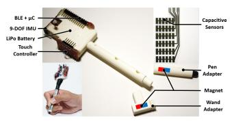
Figure 4. TMotion prototype and breakdown of its components. Permanent magnet and 9DOF-IMU are embedded for 3D position tracking.
