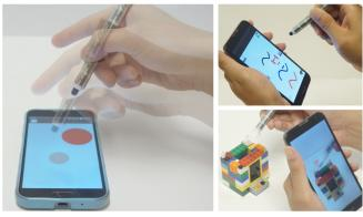
Figure 1. TMotion enables a real-time 3D position tracking using embedded permanent magnet and IMU with existing mobile device. TMotion provides interaction spaces above and behind the device while supporting discrete and continuous interactions.
